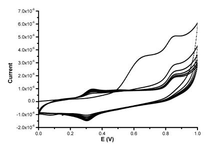
Figure 2. CV of polyaniline formed electrochemically on poly(dG)-poly(dC) DNA modified Au electrodes (see Materials and Methods) between 0–1 V vs. Ag/AgCl at scan rate of 50 mV/s in 50 mM sodium acetate buffer (pH = 3.8).
