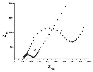
**Figure 1.** Nyquist-diagram ( $Z_{im}$  vs.  $Z_{re}$ ) for the AC impedance measurement of modified Au electrode in 5 mM [Fe(CN)<sub>6</sub>]<sup>-3/-4</sup> and 0.05 M KCl with ATPh as anchoring group (a) before and (b) after DNA immobilization.
